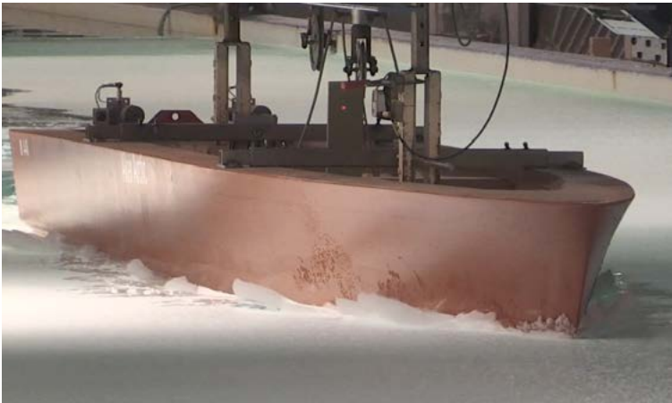
Model tests are carried out to ensure that the hull shape is suitable for icy conditions.
